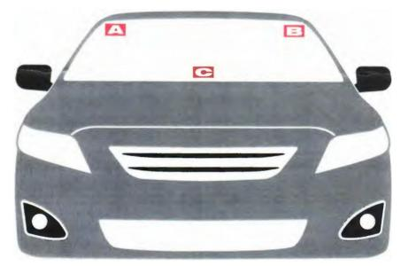
C: Some vehicles have metallic or solar windshields that require tags to be mounted in an area where those elements are removed. If the vehicle has one of these cutouts, the tag must be placed in the cutouts, (cutout location varies, see vehicle manual) or a headlamp tag must be used
